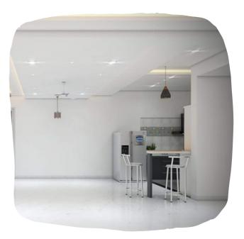
BSNZ Company produced hydrated calcium sulfate boards, often known as plasterboards, are used to create artificial ceilings. The thicknesses of these boards range from 9 to 15 mm, and they are commonly made in 4 x 6 feet, 4 x 8 feet, and 4 x 10 feet measurements. Cutting them to the right size and fitting them onto a metal structure suspended from the ceiling is an easy installation process.
